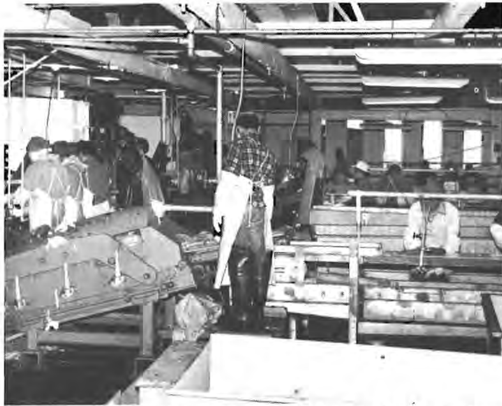
This is one of the stages in processing fish in the canneries. Fresh fish go from the "iron chinks" (so-called because such machine has taken over Chinese labor) to the cutting and gutting out of entrails. From the machines in the picture, fish are cleaned out before they are processed and packed in cans.
